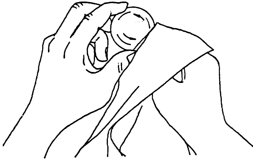
Figure 9-28. Proper Method of Holding a Lens
